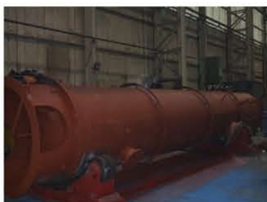
15mtr 3 Chilled buffer vessel PD5500 Cat 2 ready for hydrotesting, then insulating.
