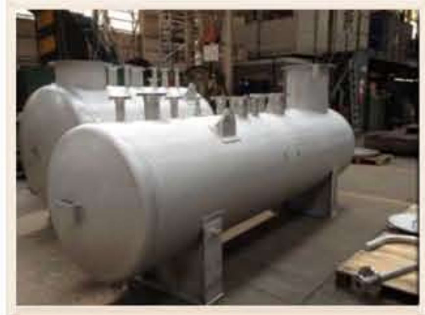
Two off 316L Stainless Steel Cylindrical Horizontal Tanks completed, part of a 16 tank order.
