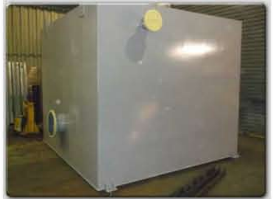
Carbon Steel Painted internally stiffened oil tank ready for delivery.
