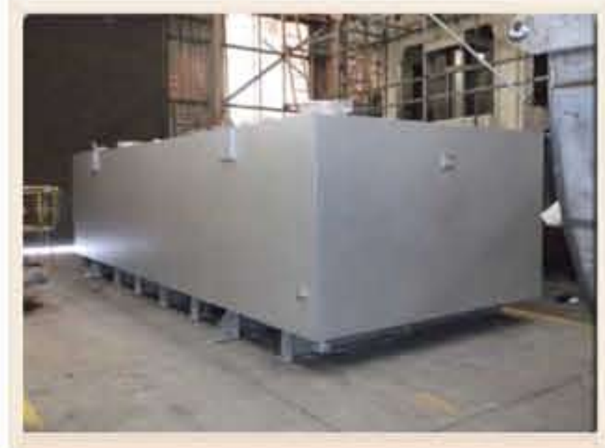
37mtr 3 - 316L Stainless Steel Rectangular internally stiffened chilled water tank ready for dispatch, insulation was carried out on site in situ.
