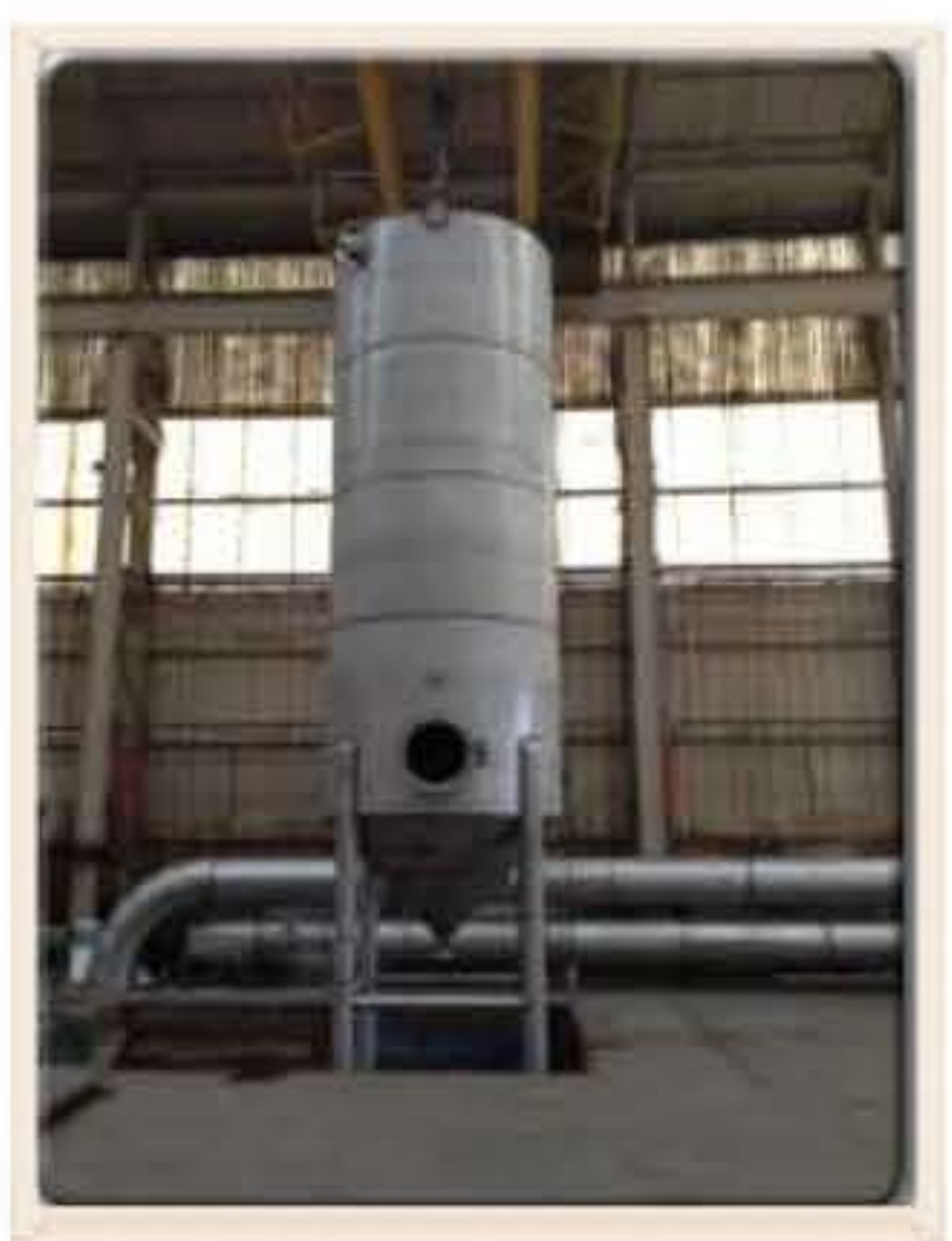
35mtr 3 Vertical Cylindrical 316L Stainless Steel tank ready for static water test in works.
